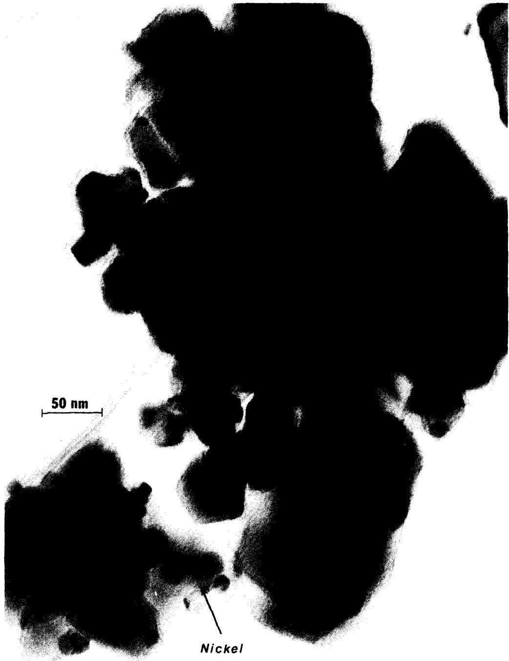
FIG. 10. Electron micrograph of sintered 15% Ni/TiO 2 .
