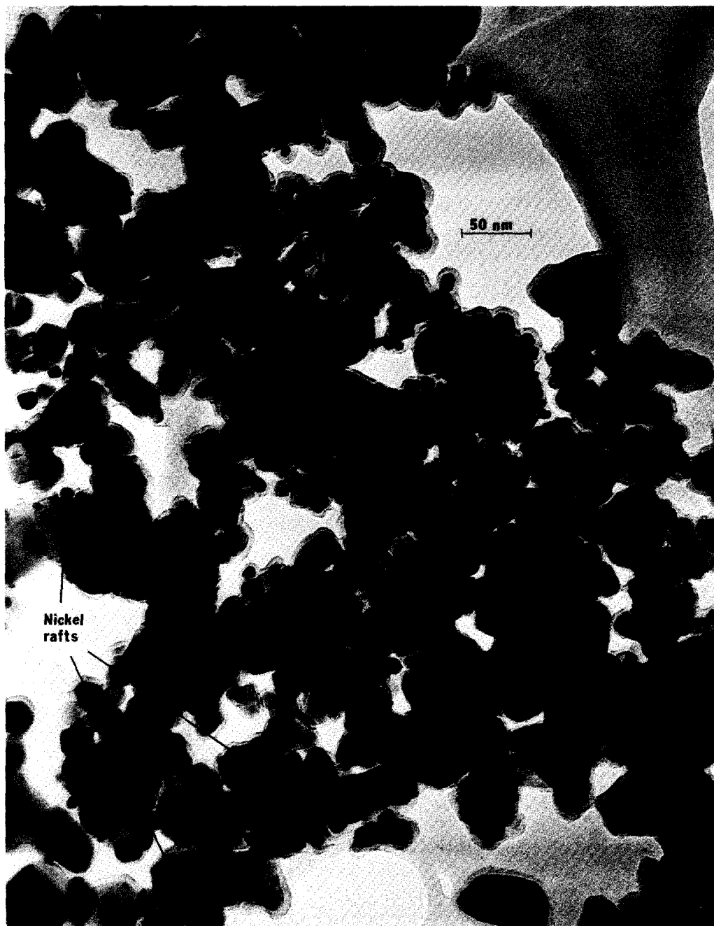
FIG. 9. Electron micrograph of 15% Ni/TiO 2 .
